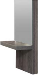
Mirror with Shelf 6mm thick mirror glass, with safety backing, bonded to timber backpanel. With shelf in matching finish. Fitted to the wall with hook battens.
